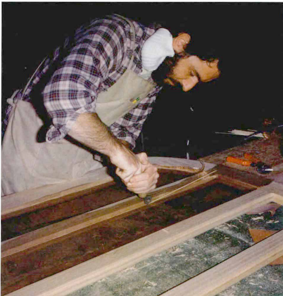
The screen is installed with the use of a splining tool. The tool consists of a handle with a metal wheel on either end, one with a convex edge and the other with a concave edge. To install the screen, the author presses the screen into the screen groove with the convex wheel. That done, he flips the tool over and presses a \frac{1}{8} -in. dowel into the groove with the concave wheel (photo above), locking the screen into the groove. Excess screen is trimmed off at the corner of the rabbet with a utility knife.
